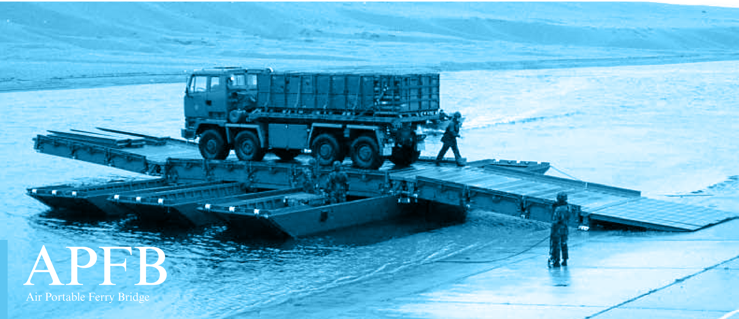
Above: Pictured here in the ferry role at MLC 35; Below: Used in an emergency relief operation.
